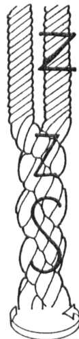
Figure 21.7 Opposing directions of singles and folding twist in a two fold yarn (S on Z). Source: Wood, 2006.
