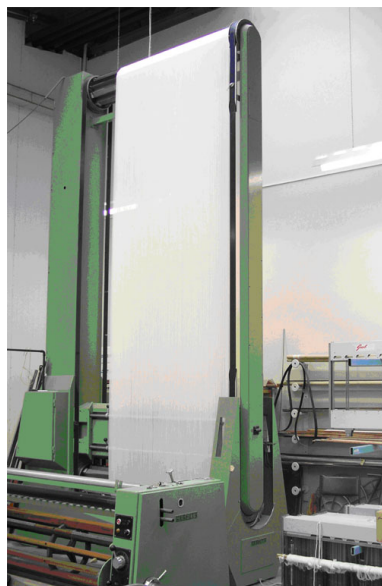
Figure 17.8 Hergeth single end warper. Photograph supplied by E. Wood courtesy Canesis Network Ltd.
