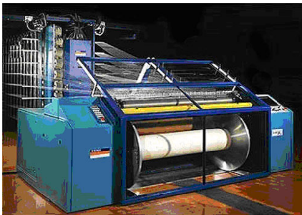
Figure 17.7 Direct winding from a creel onto a warp beam. Source: Benninger AG.
