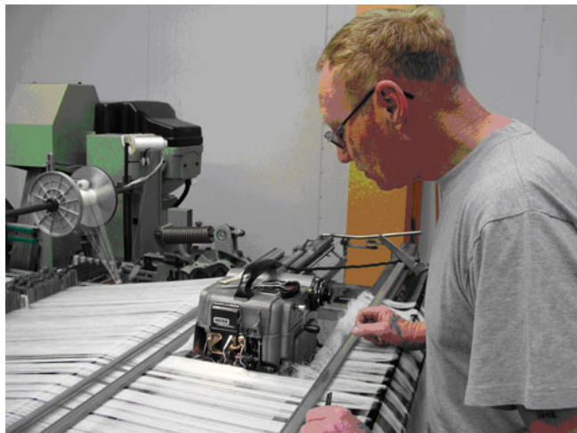
Figure 17.9 Use of a knotting machine to tie in warp yarns. Photograph supplied by E. Wood courtesy Canesis Network Ltd.
