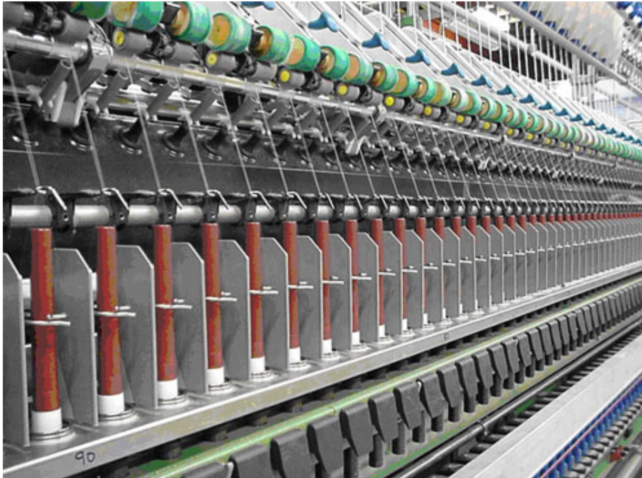
Figure 16.1 Ring spinning. Source: CSIRO TFT.
