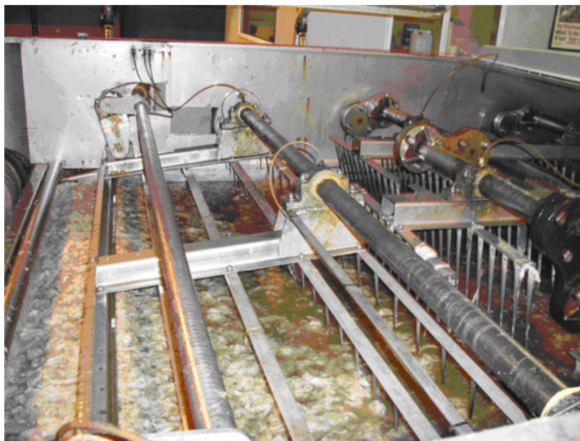
Figure 3.7 Immersed wool being moved by the rakes in a scouring bowl. Photograph supplied by E. Wood, courtesy Canesis Network Ltd.
