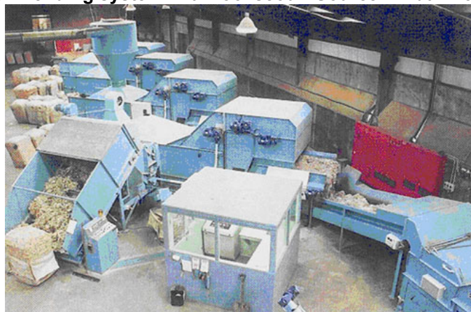
Figure 3.5 Blending system in a wool scour. Source: Andar Holdings Ltd.
