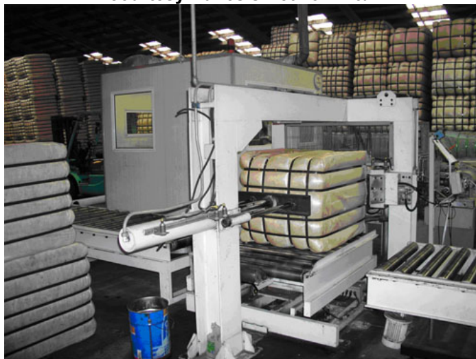
Figure 3.9 Core sampling of a high density bale. Photograph supplied by E. Wood, courtesy Canesis Network Ltd.
