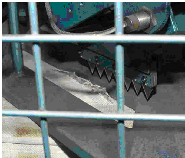
Figure 7.2 Pack slitter automatically cuts grab hole in pack with sharp blades. Source: AWTA, (2005).
