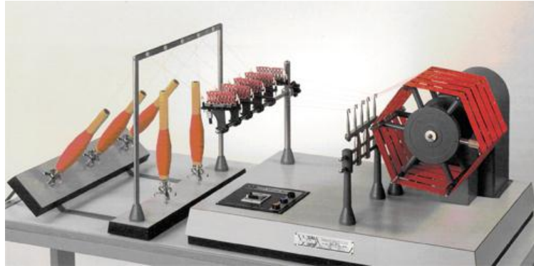
Figure 15.1 Wrap reel for yarn length measurement. Source: James H Heal & Co Ltd. (1994).
