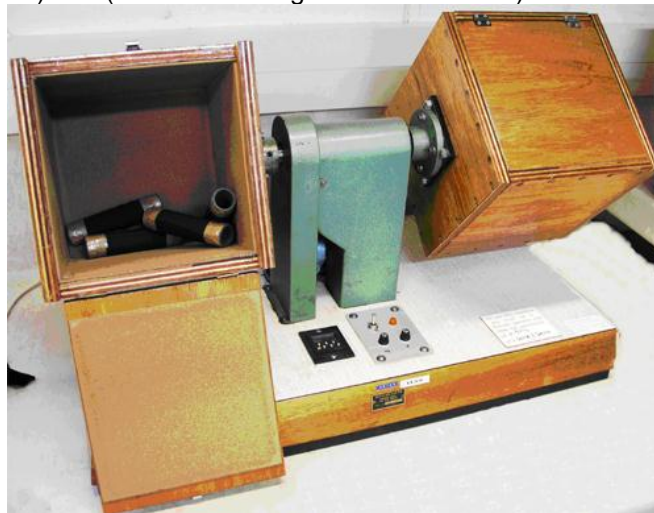
Figure 15.11 Pilling box opened to show fabric specimens on tubes.
