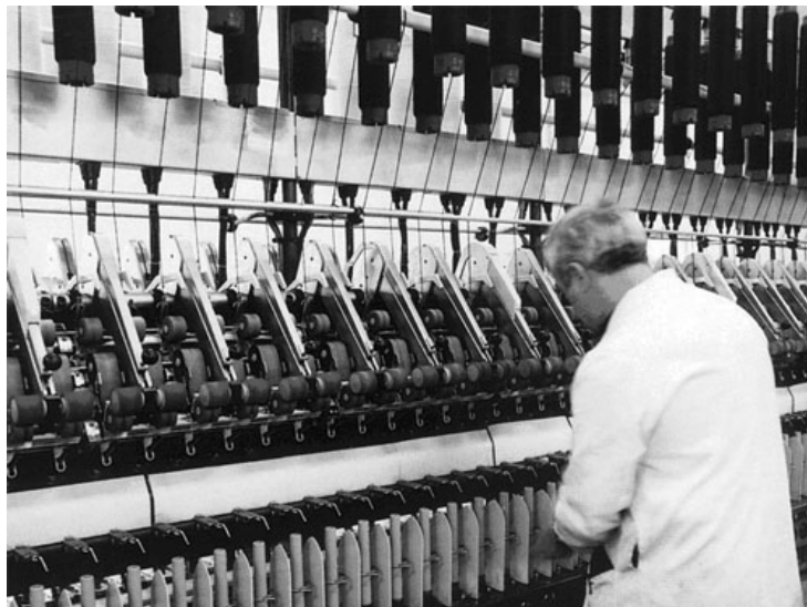
Figure 1.12 Worsted spinning frame. Source: Wood, 2006.
