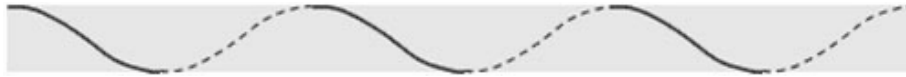
Figure 1.13 Helical path of a fibre in an ideal worsted yarn. Source: Wood, 2006.
