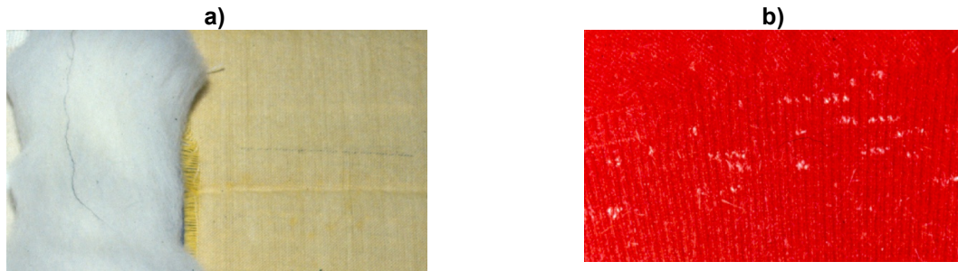
Figure 4.4: a) Black hay bale twine in top and woven fabric and b) white poly bag fibres in knitted fabric (Vern Gibbs PIRSA)
